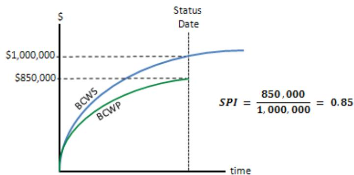
Figure 1. SPI Example
