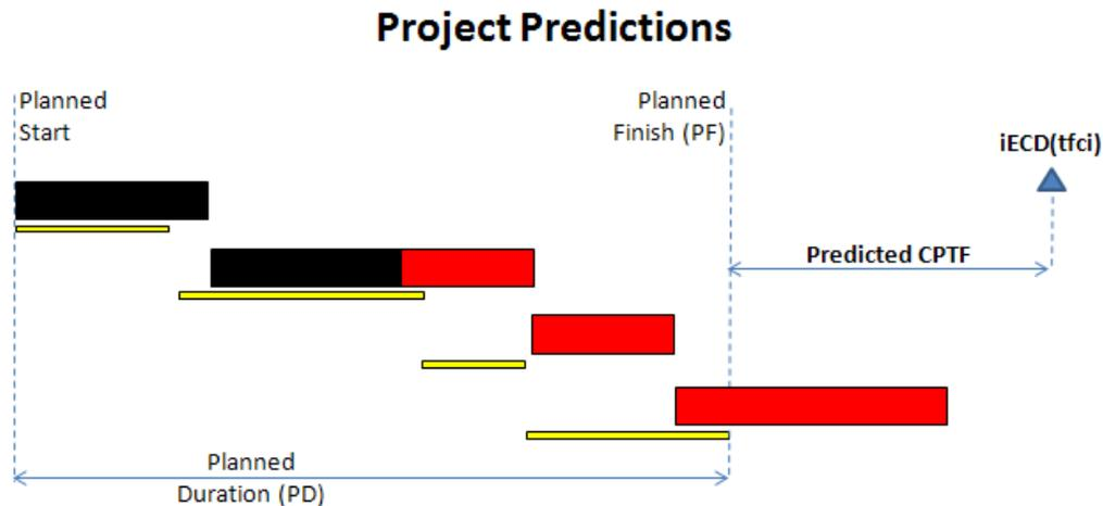
**Figure 9. Predicted Project Completion Based on TFCI**
