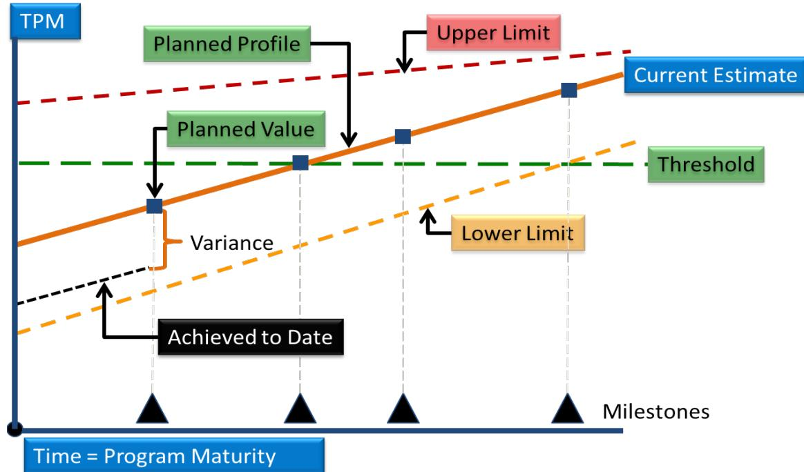
Figure 35. Plotting the Progress of TPMs against KPPs
