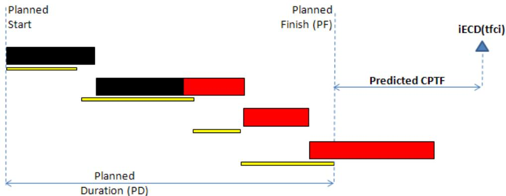
**Figure 9. Predicted Project Completion Based on TFCI**
