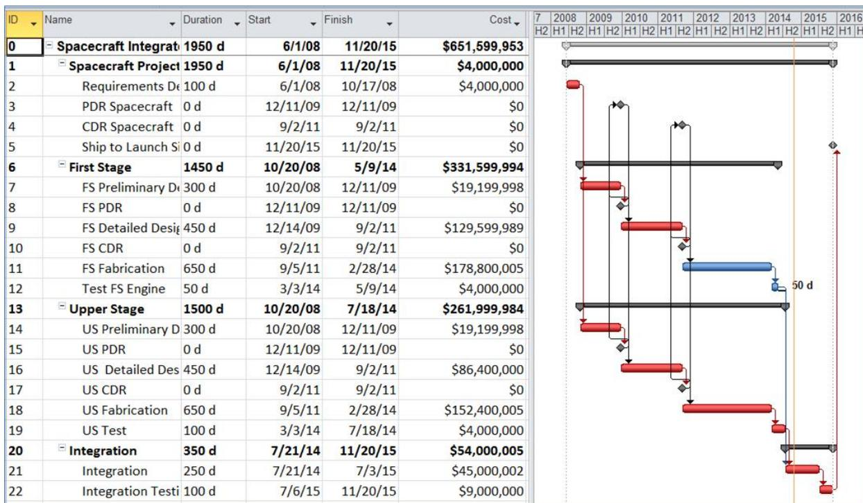
This is a project starting June 1, 2008, with a ship to launch site end date of November 20, 2015. The project cost is estimated at \$651.6 million.<sup>2</sup> Resources are shown on the bar chart and include mostly labor, with some equipment in the First Stage and Upper Stage Fabrication activities.
